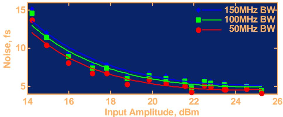
Figure 8: CTF3 results, noise in femtoseconds of the detection hardware, including LO generation, down-mixing and IF detection. The beam pickup and the timing reference for LO generation were common to the system.
