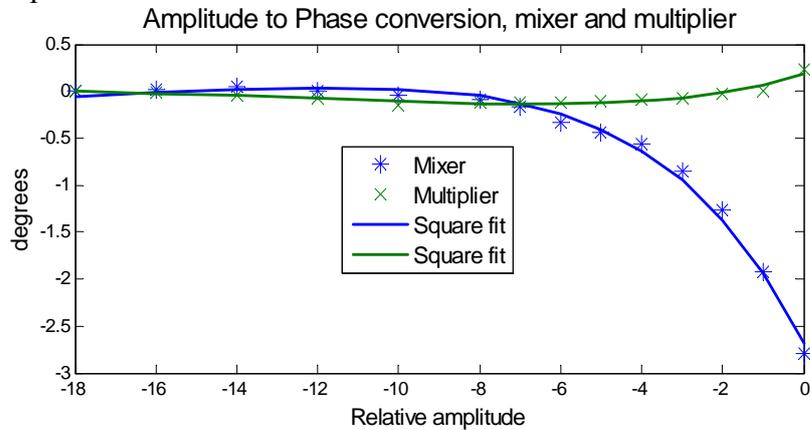
**Figure 2: Amplitude to phase conversion when mixing to baseband in a phase detector. The better performance of the multiplier indicated its suitability to the task.**
