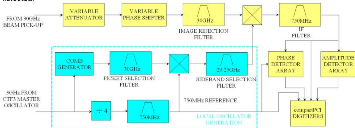
Figure 5: LO generation, down-mixing and detection
