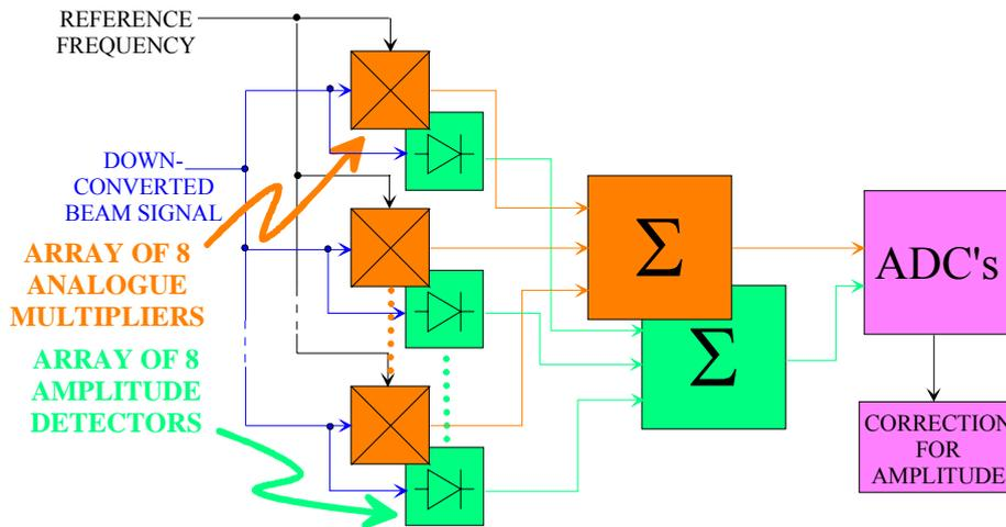
Figure 4: Arrays of multipliers and amplitude detectors
