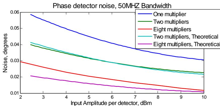
**Figure 3: Improved signal to noise ratio resulting from the use of arrays of devices**
