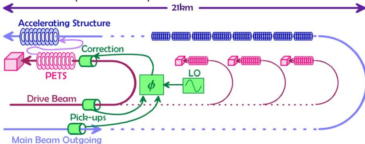
**Figure 1: Phase detection scheme for CLIC. The outgoing main beam and the drive beam are both measured with respect to a local oscillator. These measurements provide a signal for the correction prior to the Power Extraction and Transfer Structure.**
