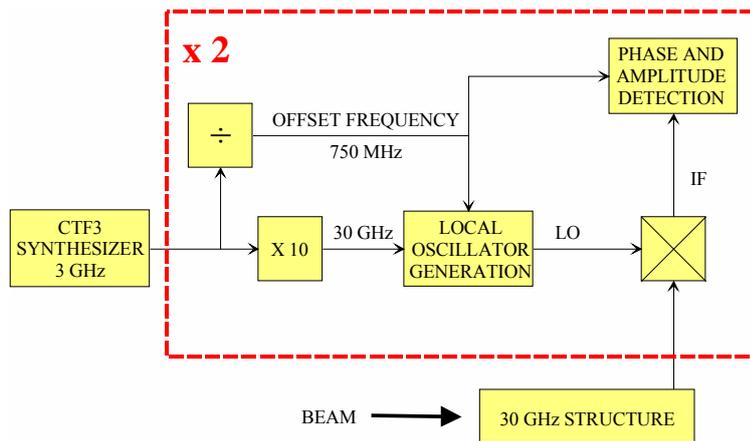
Figure 6: CTF3 test setup. Two systems are compared to each other.
