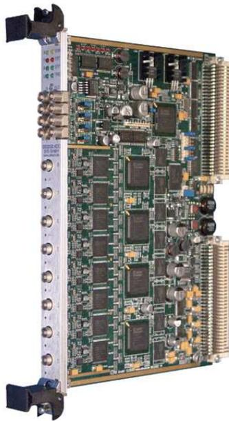
Figure 9: SIS3001 digitiser module (without the protective lid).
