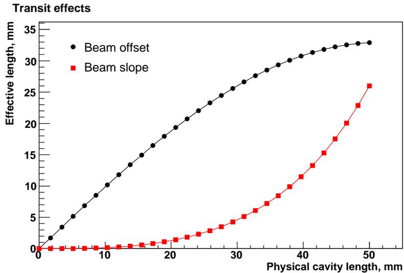
Figure 1: Effective cavity length for the position and incline contributions to the dipole mode vs. physical cavity length.
