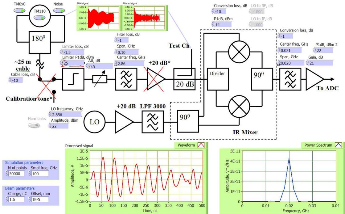
Figure 8: BPM processor schematic built into simulation program interface.
