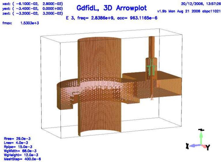
Figure 3: Inside structure of the reference cavity.
