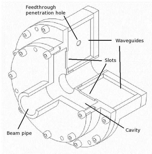
Figure 4: A 3D sketch of the model cavity.
