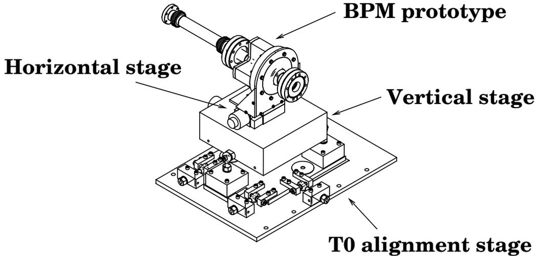
Figure 7: BPM prototype in assembly with the support stand, vertical and horizontal mover stages mounted on an adjustable supporting platform (T0 stage).
