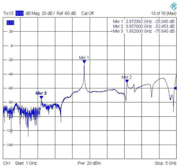
Figure 5: Frequency scan with an external antenna, marker 1 shows the dipole mode peak, marker 2 - second monopole, marker 3 - first monopole.
