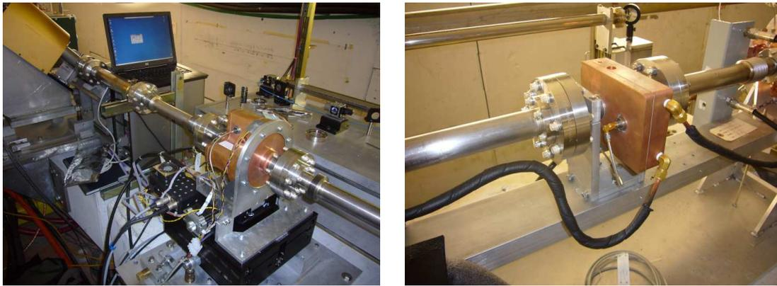
Figure 6: Vacuum prototypes of the position (left) and reference (right) cavities in the End Station A beamline.
