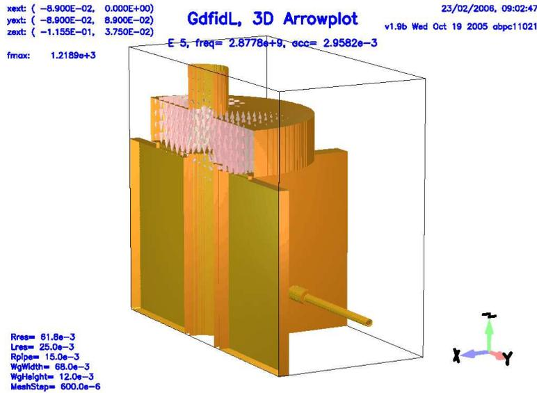
Figure 2: Dipole mode fields shown schematically as generated by GdfidL.
