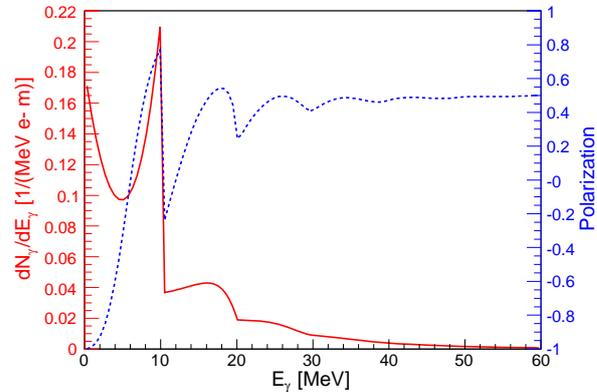
Figure 1: Energy distribution and polarization of photons generated by an electron passing one meter of the undulator (period is 1.15 cm and K value is 0.92).
