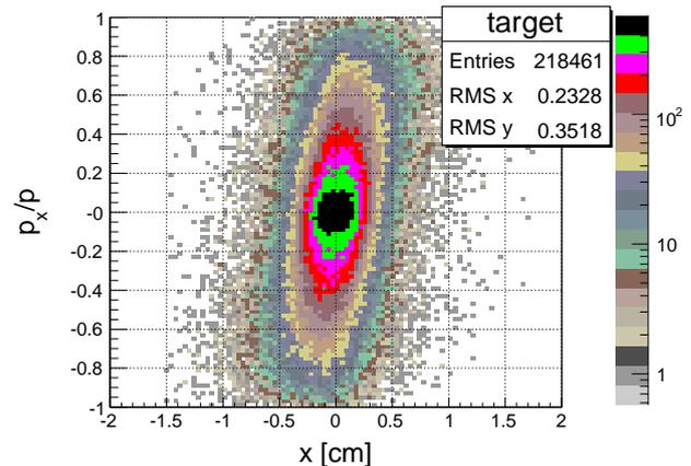
Figure 2: The positron  $xx'$  phase space after the target calculated by FLUKA for  $10^7$  primary photons.
