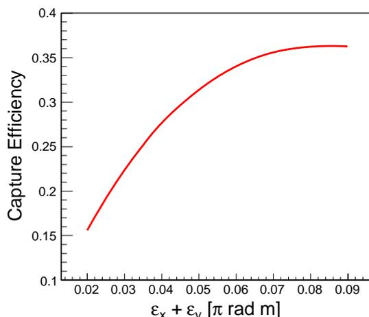
Figure 7: Positron capture efficiency vs cut on transverse edge emittance (after applying 10 mm longitudinal bunch length cut) at the 125 MeV point of positron preaccelerator.
