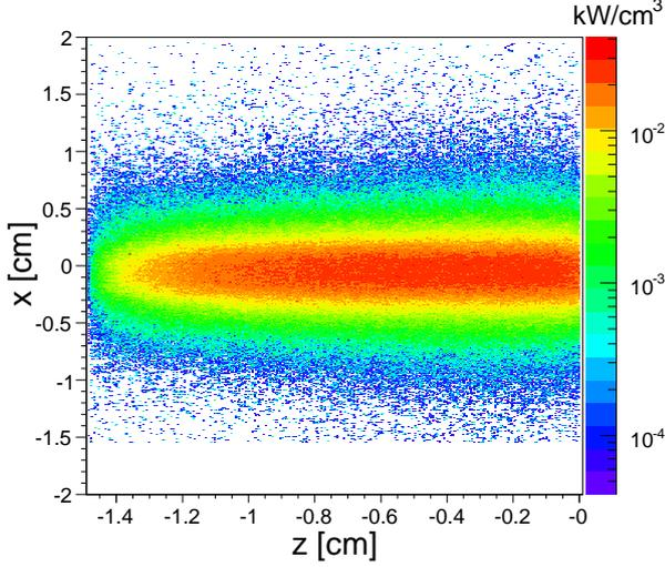
Figure 3: The power deposited in the target by 117 kW photon beam (FLUKA).
