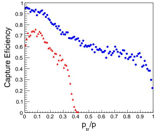
Figure 6: Positron capture efficiency vs normalized transverse momentum  $p_{tr}/p$  at the 125 MeV point of positron preaccelerator: blue circles – without cuts; red triangles – with a longitudinal bunch length cut of 10 mm and a transverse diagonal emittance cut of  $0.04 \pi$  rad m.
