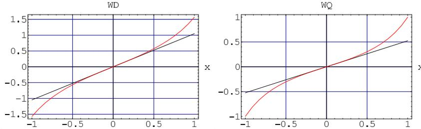
Figure 1: Dipole (left) and quadrupole (right) components of the wake field as a function of  $x_0/g, x = 0$  and  $x_0 = 0, x/g$  respectively, for  $y, y_0 \ll g$ . The fully nonlinear expressions (red lines) are compared with their linear approximations for  $x_0, x \ll g$  (black lines).
