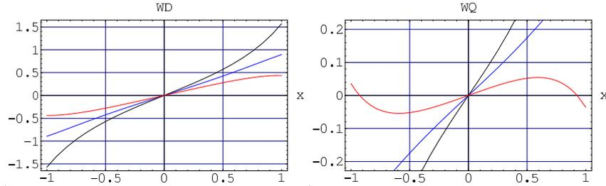
Figure 2: Dipole (left) and quadrupole (right) components of the wake field as a function of  $x_0/g, x = 0$  and  $x_0 = 0, x/g$  respectively, for  $(y - y_0)/g = 0$  (black), 0.5 (blue), 0.8 (red).
