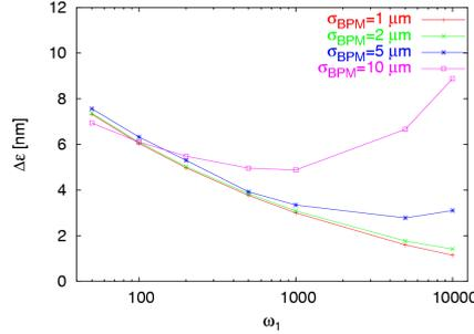
Figure 4: Final emittance growth for an ILC main linac in the laser-straight configuration, as a function of the DFS weights  $\omega$ , for different BPM resolutions. A final emittance growth of about 2 nm is well under the design limits.
