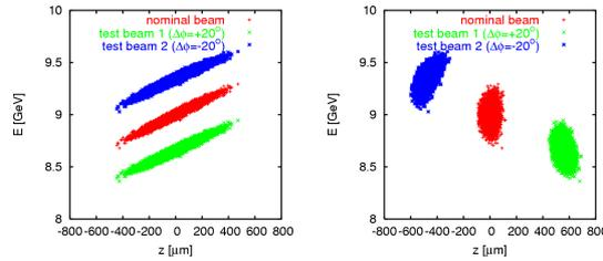
Figure 1: Longitudinal phase space of off-phase bunches at the entrance (left) and at the exit (right) of the magnetic chicane of the CLIC bunch compressor stage 2.
