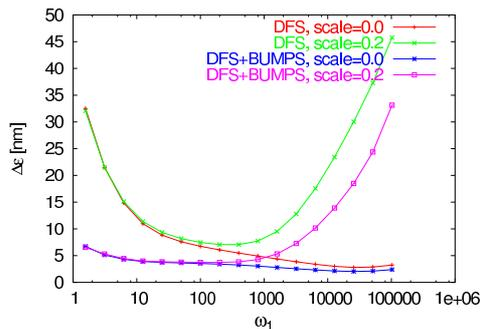
Figure 5: Final emittance growth for an ILC main linac that follows the Earth’s curvature, as a function of the DFS weights  $\omega$  and in presence of bpm scale errors. Bpm scale errors become relevant for high weights, where DFS is no longer enough to maintain the emittance under acceptable limits and one needs to use further optimization procedures.
