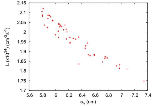
Figure 6: Luminosity versus the combined vertical beam size of both  $e^-$  and  $e^+$  beams at the IP. Feedback simulation carried out for  $e^+e^-$  collisions under the effect of the missalignments produced by the ground motion after 1 s.
