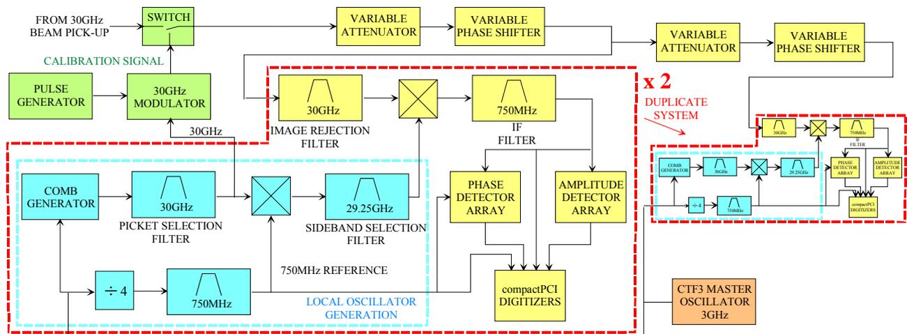
Fig. 1 Set-up for beam tests in CTF3.
