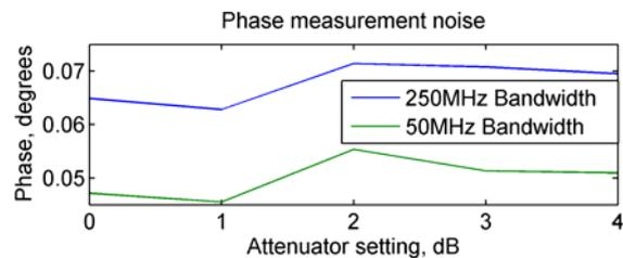
Fig. 3 Jitter of beam phase measurement system.
