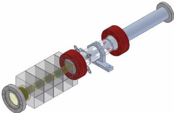
Figure 3: T488 module design showing (left to right) material mockup of the mask, beamline calorimeter, BPM, and magnet.
