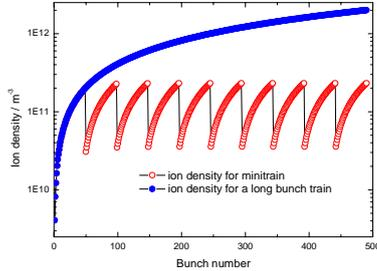
Fig. 3: Ion density versus bunch number for 10 bunch trains in fill pattern case A.
