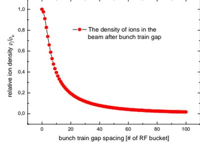
Fig.1: The density of the residual ions in the beam after the bunch train gap.
