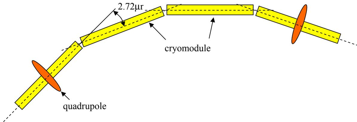
**Figure 1: Sketch of Earth curvature following linac geometry**
