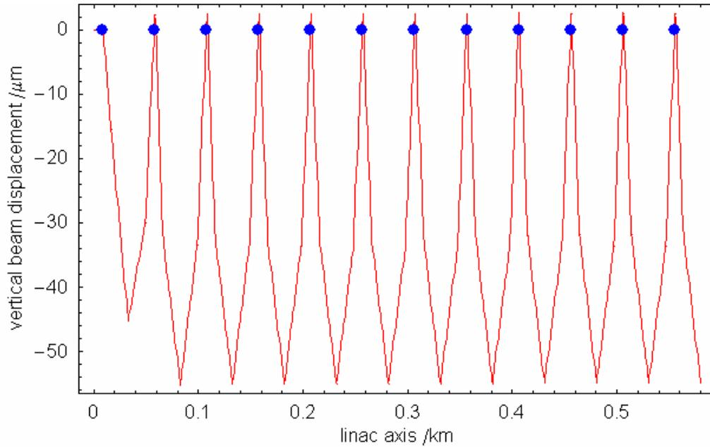
**Figure 2:** Design orbit relative to the curved geometry of a section of linac which follows the Earth's curvature. The blue dots correspond to the BPM locations (zero by default after steering).
