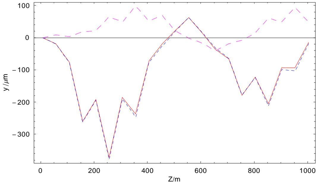
Figure 7: Effect of wakefield on off-energy trajectory for the first 40 quadrupoles. The red solid line is the result of tracking a single particle representing the bunch centroid (no wakefields), as used in the reported simulations; the blue dashed line is the simulation of the full bunch including wakefields; and the magenta dashed line is the difference ( $\times 10$ ).
