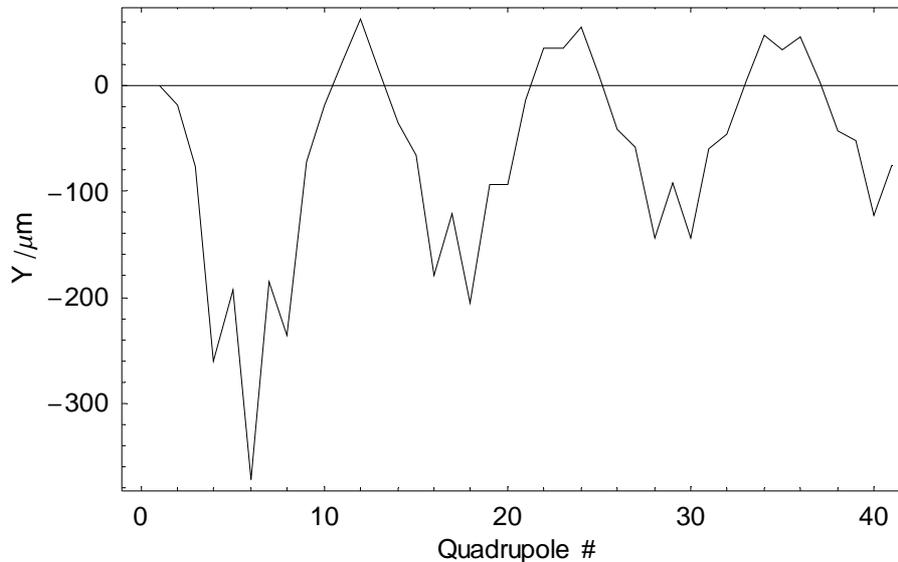
Figure 3: Example of the design dispersive orbit (first segment of 40 quadrupoles), for an initial energy change of -20% (only BPM locations shown)
