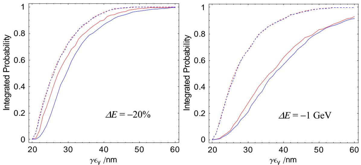
**Figure 5: Simulations results of 1000 random 250 GeV linacs. The graphs indicate the fraction of the seeds resulting in less than or equal to the specified emittance. Red and blue lines show the results for the laser-straight and curved geometries respectively. Solid lines indicate the as calculate projected emittance, while the dashed lines show the emittance after removing the linear momentum correlation.**
