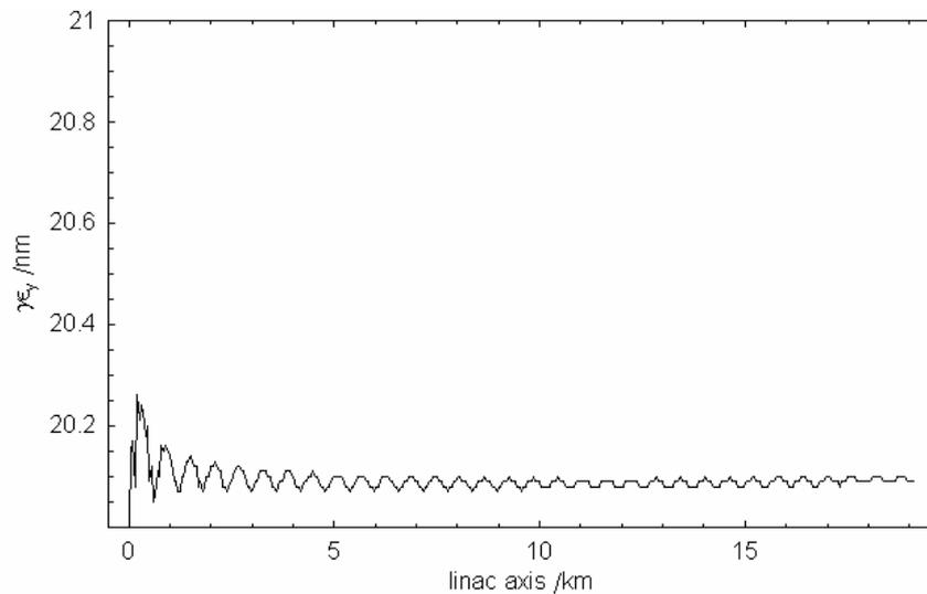
**Figure 4: Design emittance for a perfect linac following the Earth's curvature.**
