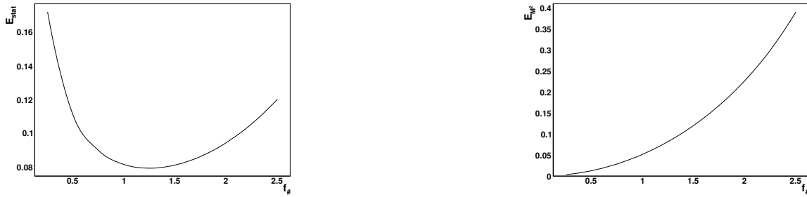
Figure 12: (a): Statistical error E_{\text{stat}} , (b): laser error E_{M^2} for \xi = 1 (Eq. 32) using N_{\text{scan}} = 19 scan points versus the f -number of the final focus lens, using a laser with M^2=1.3 and operating in the TM_{00} mode with \lambda = 532 nm. The electron bunch is assumed to have a Gaussian transverse profile with \sigma_{ey} = 1 \mu\text{m} and \sigma_{ex} = 25 \mu\text{m} .
