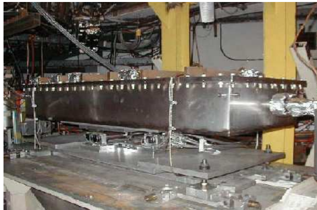
Figure 6: Mover box at ESA for measurements of beam kick factors from wakefield measurements induced by different collimator designs.
