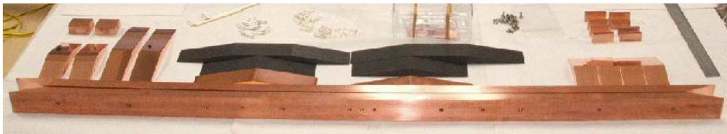
Figure 3: Produced collimator jaws for wakefield measurements. The longest pair of collimators is shown in the front of the picture and has a length of 1m.
