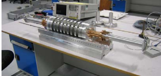
Figure 1: Picture of the bench-top experimental model of the modular crab cavity.
