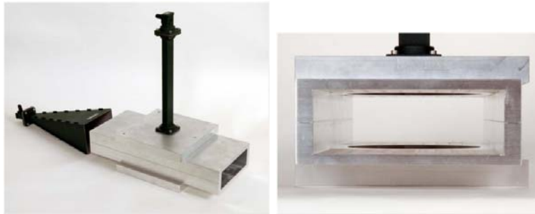
Figure 5: Photographs of the nearly-confocal resonator prototype installed onto a rectangular Aluminium pipe with a standard M-band waveguide connected to the upper mirror.
