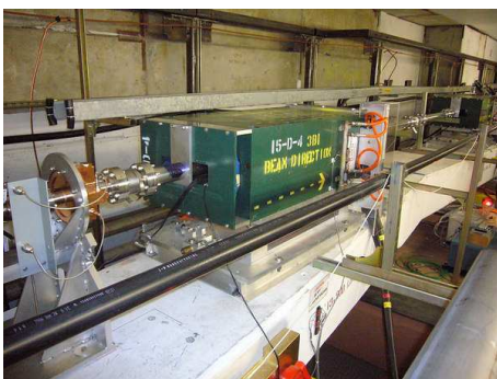
Figure 4: The first chicane magnet and BPM5 in the ESA beamline.
